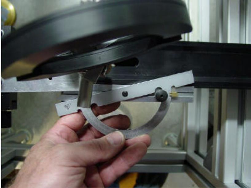
22. TIMMI2 has to be put horizontal as well. Check with the precision level that the ribs of the front flange are perfectly horizontal. The adjustment can be done with a 13mm wrench on the base of the Bosch structure.
