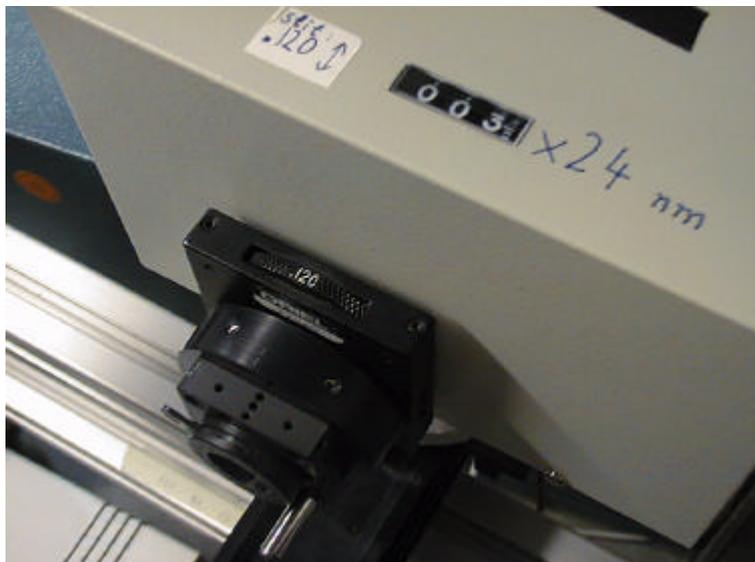
55. Set up TIMMI for through-slit imaging mode:
