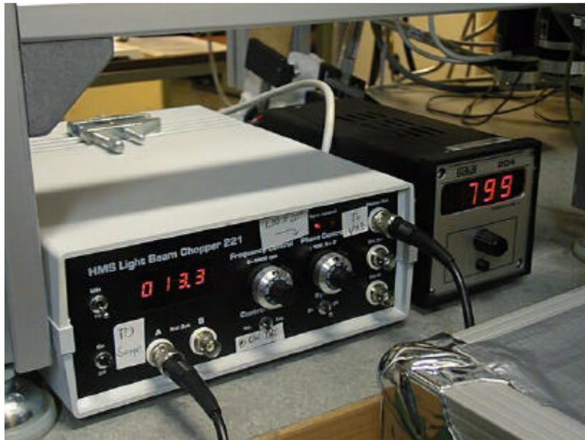
12. Adjust the frequency control such, that on the scope the two traces are almost the same frequency. Don't care if one of the signals (the un-triggered channel) is leading or lagging.
