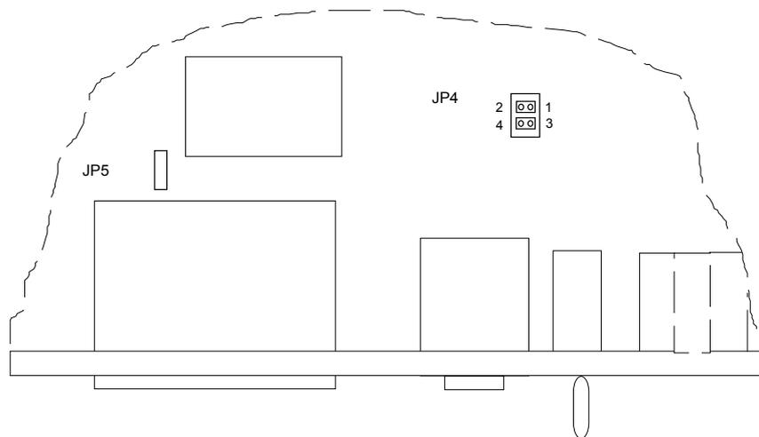
Fig. 4. JP4 and JP5 jumper pin numbering.
