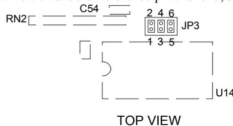
Fig. 3. JP3 jumper pin numbering.
