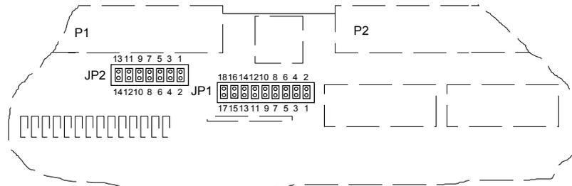
Fig.2. JP1 and JP2 jumper pin numbering.
