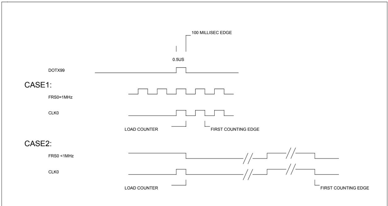
Fig. 8 Timing for 'gate next 100 millisecond'.
