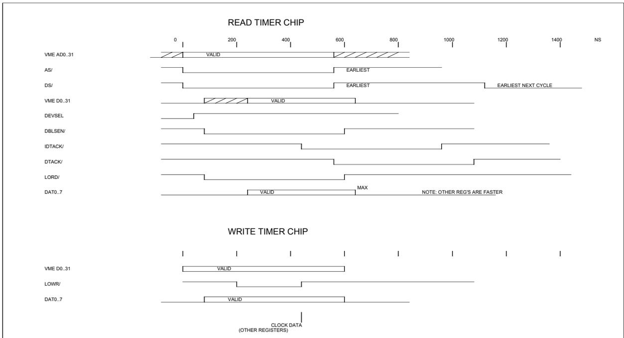
Fig. 7 VME read / write timing.
