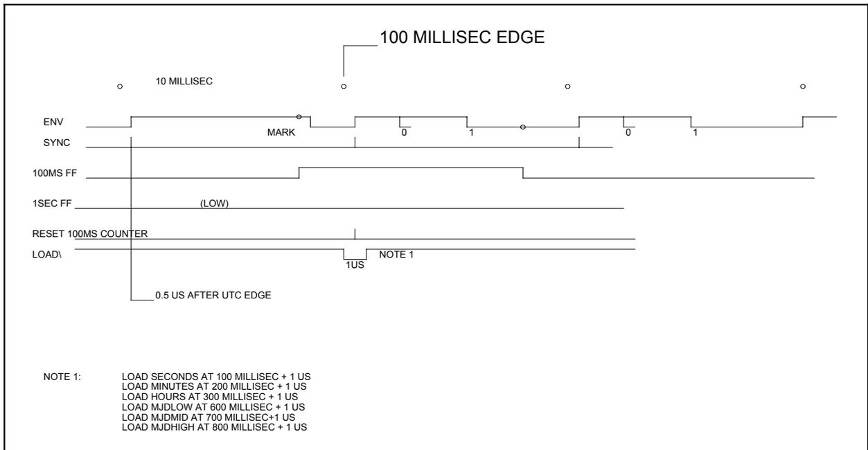
Fig. 11 UTC 100 millisecond decoding.
