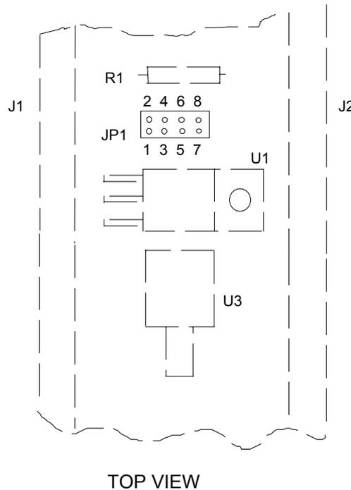
Fig. 5. TIM Backplane Receiver JP1 jumper pin numbering.
