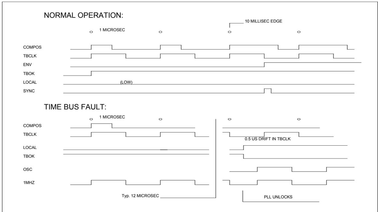
Fig. 9 UTC composite decoding.
