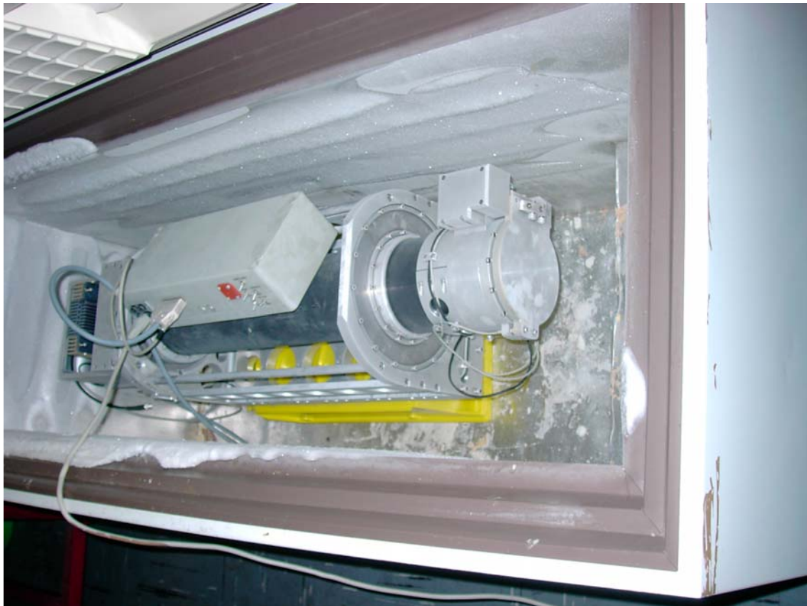
Figure 3 : APT in the freezer after 12 hours at -33°C
