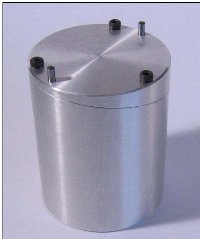
Figure 10: Closed Block Ready for Machining
